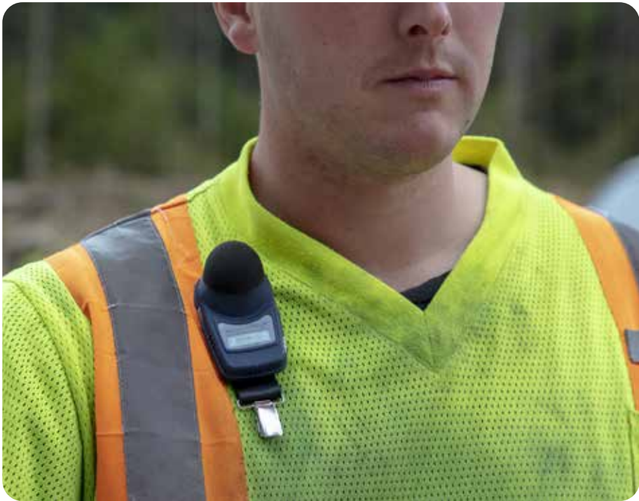
Workers wear noise dosimeters over the shoulder or on the collar.
