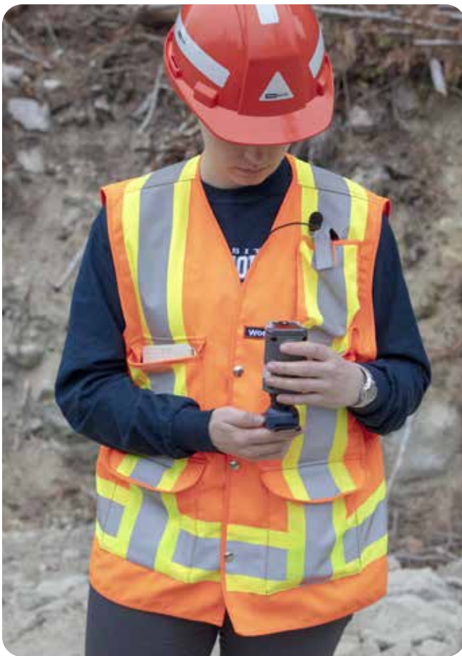
Meters must be calibrated before and after a survey.
